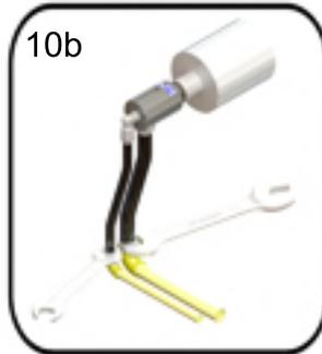
10. Connect hoses to the supply and return lines. Use flexible hoses and never install joint directly to the pipes.
