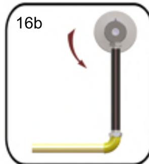
16. Flexible hoses must not be twisted during operation. Use proper pipe fittings.
