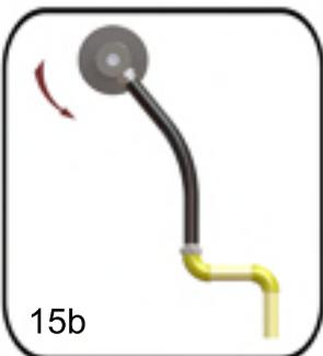
14. Flexible hoses must not be twisted during operation. Twisted hoses lose flexibility.
