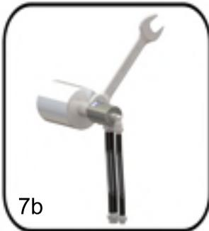
9. If the joint shaft is quick release; put a new copper washer into the bore of the roll, assemble qr flange onto the shaft, place split rings onto the socket on the shaft correspondingly, place qr flange onto the split wedges and fix the flange to the bore of the roll with appropriate bolts.
