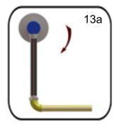
12. If rotating joint and pipe axis are not on the same axis, hose must be installed with a smooth curve.
