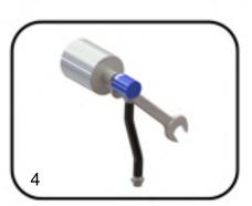
4. Apply adhesive or teflon tape to the thread of the shaft and install the joint to the machine. When installing, pay attention not to install eccentrically.
