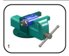
1. First hold the housing of the joint with a bench wise. Do not clamp too tightly, it will damage housing or bearings.
