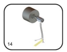
1. First hold the housing of the joint with a bench wise. Do not clamp too tightly, it will damage housing or bearings.
