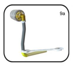
9. Connect hoses to the supply and return lines. Use flexible hoses and never install joint directly to the pipes.
