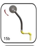
14. Flexible hoses must not be twisted during operation. Twisted hoses lose flexibility.
