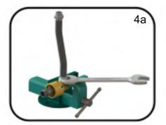
4. Apply sealant/adhesive or teflon tape to the threads of the hoses and assemble them to the housing.
