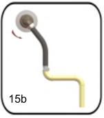
15. If rotating joint and pipe axis are not on the same axis, hose must be installed with a smooth curve.
