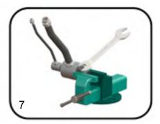
6. Rotate the shaft  $180^{\circ}$  and hold the joint from the main shaft with a bench wise.
