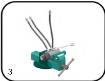
3. Place new copper gasket onto the nipple threads of the drain hose and assemble it to the drain port of the housing.
