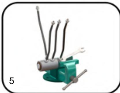
4. Hold the joint from the main shaft with bench vise.
