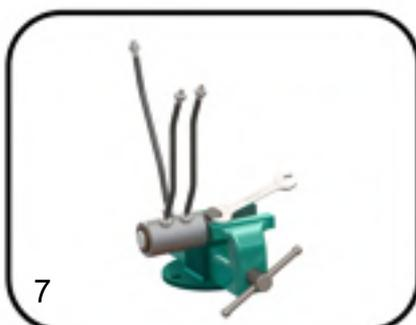
6. Rotate the shaft 180° and hold the joint from the main shaft with a bench vise.
