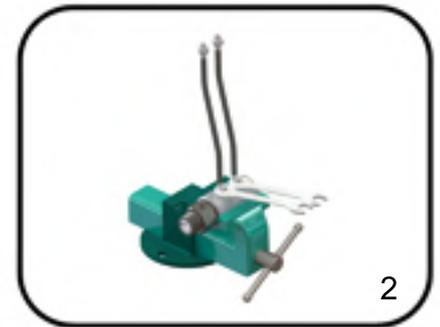
2. Place new copper gaskets onto the nipple threads of the hydraulic hoses and fix them to the ports of the housing.
