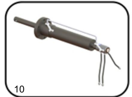
13. Rigid connection of the anti rotation rod will damage the joint.
