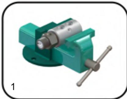
1. First hold the housing of the joint with a bench vise. Do not clamp too tightly, it will damage housing or bearings.
