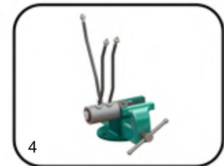
5. Place a new copper washer onto the nipple thread of the hose and fix it to the side outlet port of the shaft.
